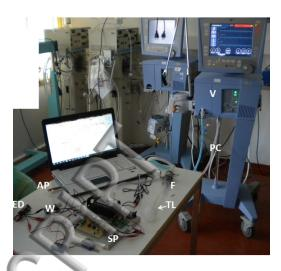
FIG. 5. Experimental setup for trials with a pulmonary ventilator with a bi-tube connection typically used in the intensive care units with wireless configuration of the Patient Ventilation Monitoring Unit. V: mechanical ventilator; Y: wye-shaped element of breathing circuit; TL: (neonatal/pediatric) test lung; P: pressure sensor; F: flow sensor (pneumotachograph); T: thermometer; ED: end device; AC: access point; SP: sensors platform; PC: patient circuit; W: wired connection between SP and ED.
